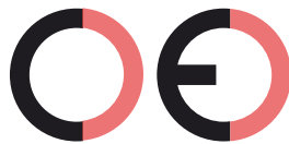
False CE Mark (too far)
